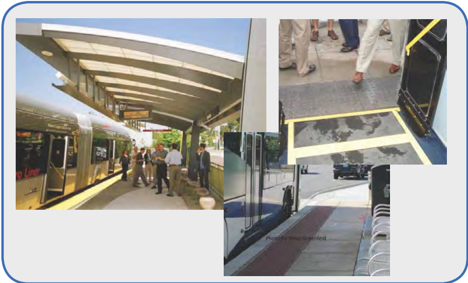
Enhanced stations are designed for passenger comfort and full accessibility, possibly including level boarding of the bus.
