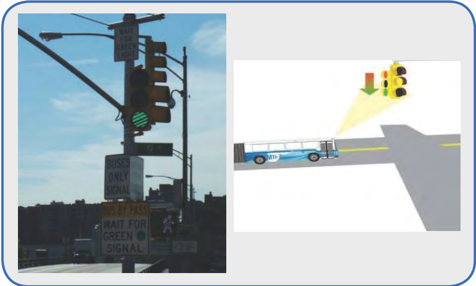
Signal priority allows for faster and more reliable travel times by giving buses extra time to move through green lights.
