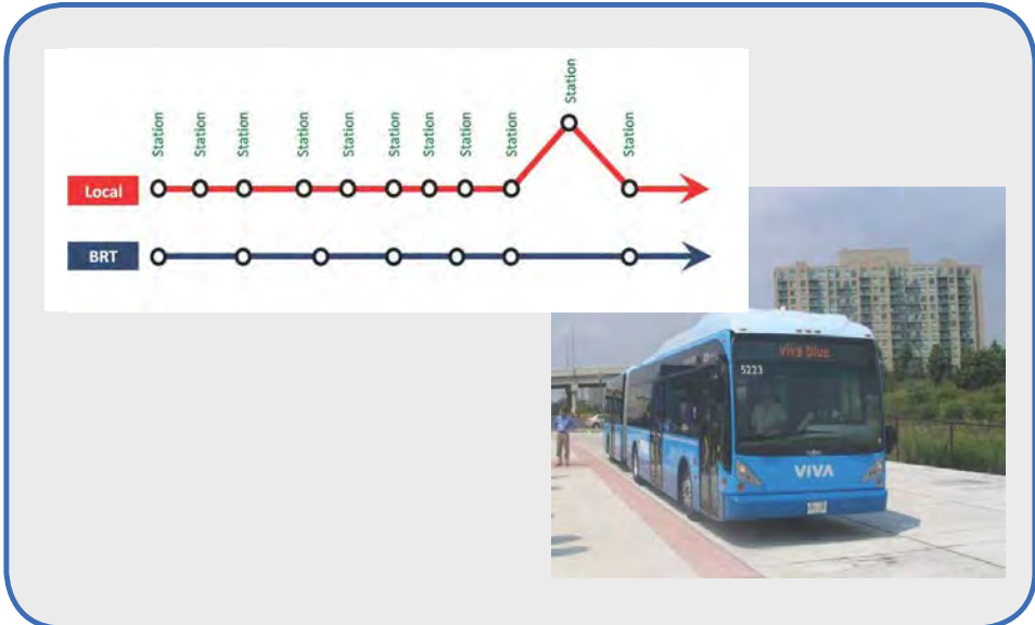
Enhanced service plans considers operating express or limited-stop services, and overall route simplification, while branding and improved vehicles creates a distinct identity for BRT.
