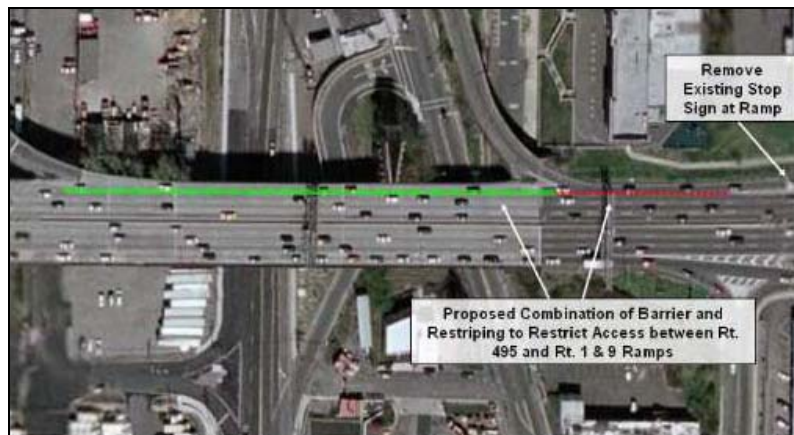
Figure 7-9c – Proposed Restrictive Barrier / Re-striping Combination
